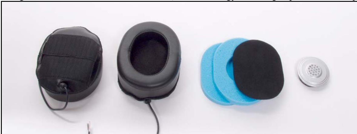
Figure 4. Gentex HGU-56/P Aircrew Integrated Helmet System earcup configuration displayed with the Oregon Aero earcup replacement products evaluated in this study. (a) Oregon Aero HushKit™, (b) Oregon Aero SoftSeal™ with Oregon Aero HushKit™, (c) Oregon Aero SoftSeal/HushKit Combo™
